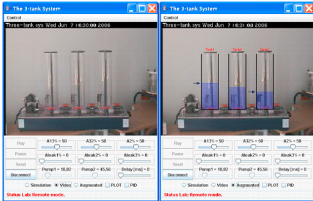
Fig. 2. The three-tank system. The laboratory combined a virtual and a remote plant and superimposed their responses.
